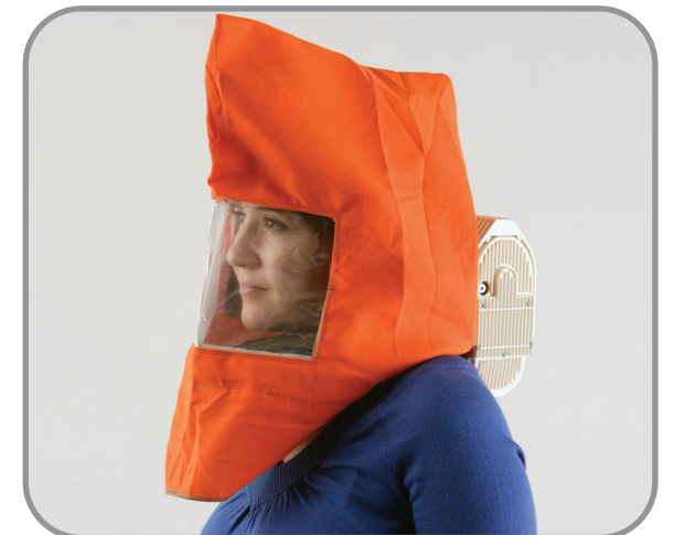
6. While standing upright, pull hood down until headband firmly engages forehead. Clear neck seal of obstructions and check neck seal for secure fit. Note: Remove when flow noise stops.
