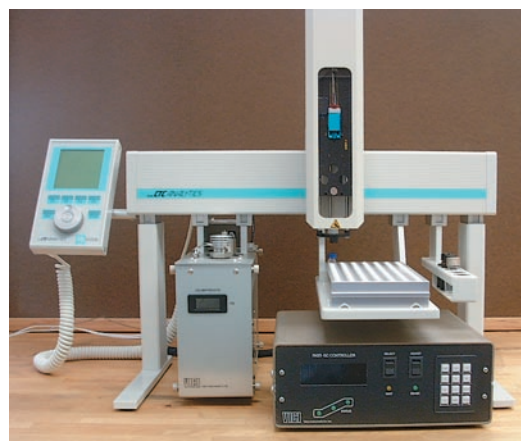
Fast GC Module and controller mounted on an autosampler
