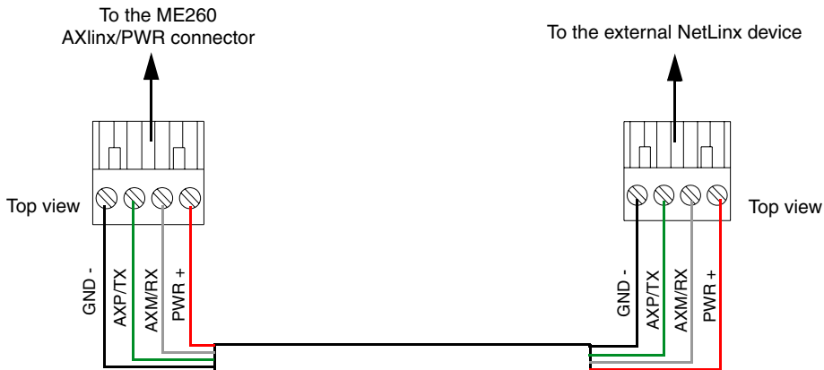
FIG. 6 4-pin mini-Phoenix connector wiring diagram (direct data and power)
