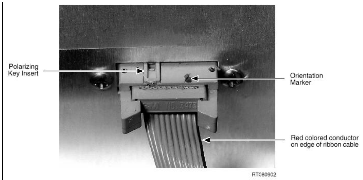
Figure 6-32 Close-up of Alarm Connector
