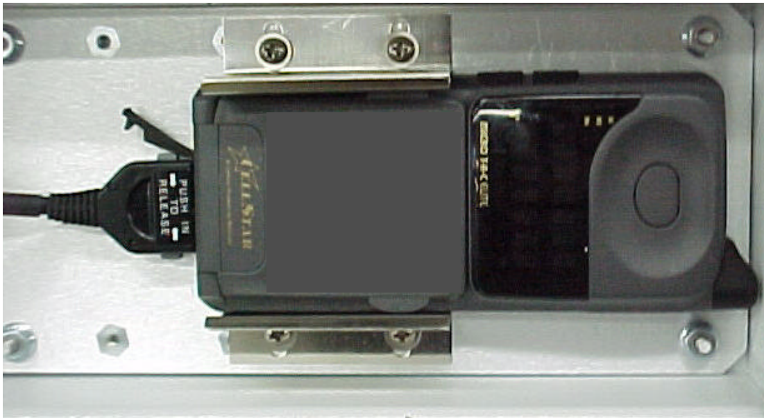
Figure 13-1 Motorola Micro T.A.C. Elite II Cellular Phone, Installed in Entry Box Lid
